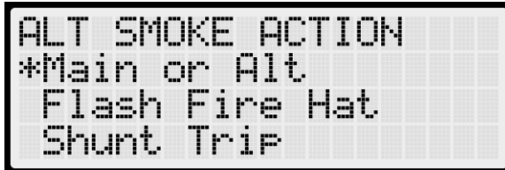
Figure 270: ALT SMOKE ACTION Menu – Main or Alt, Flash Fire Hat, Shunt Trip
