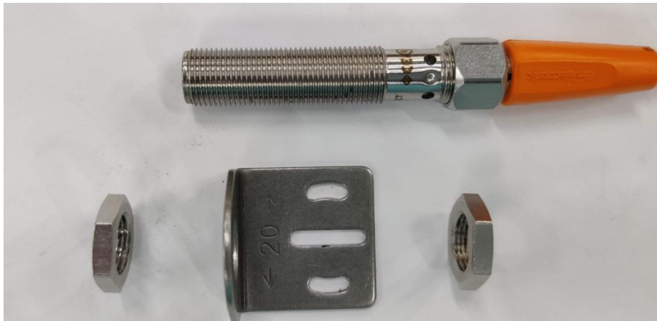
Figure 105: Proximity Sensor Assembly
