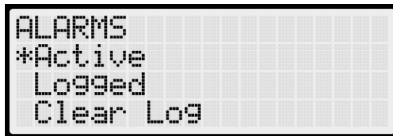
Figure 183: ALARMS Menu – Active, Logged, Clear Log
