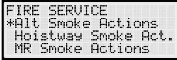
Figure 269: FIRE SERVICE Menu – Alt Smoke Actions, Hoistway Smoke Actions, MR Smoke Actions
