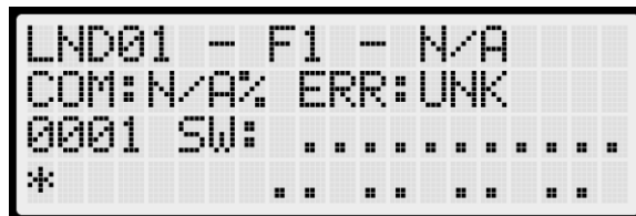
Figure 37: Uninitialized Hall Board Status
