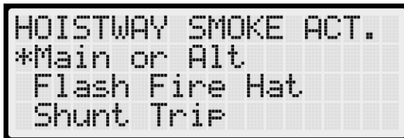
Figure 271: HOISTWAY SMOKE ACTION Menu – Main or Alt, Flash Fire Hat, Shunt Trip
