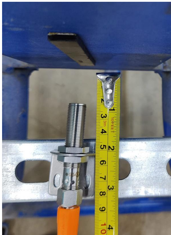
Figure 106: Mounting Proximity Sensor Assembly (Example)
